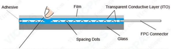
Input will be made as the top film is pressed down and the top and bottom ITO layers contact.
