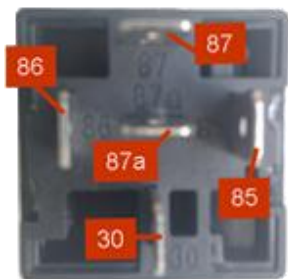
Bottom of the relay Wiring Diagram
