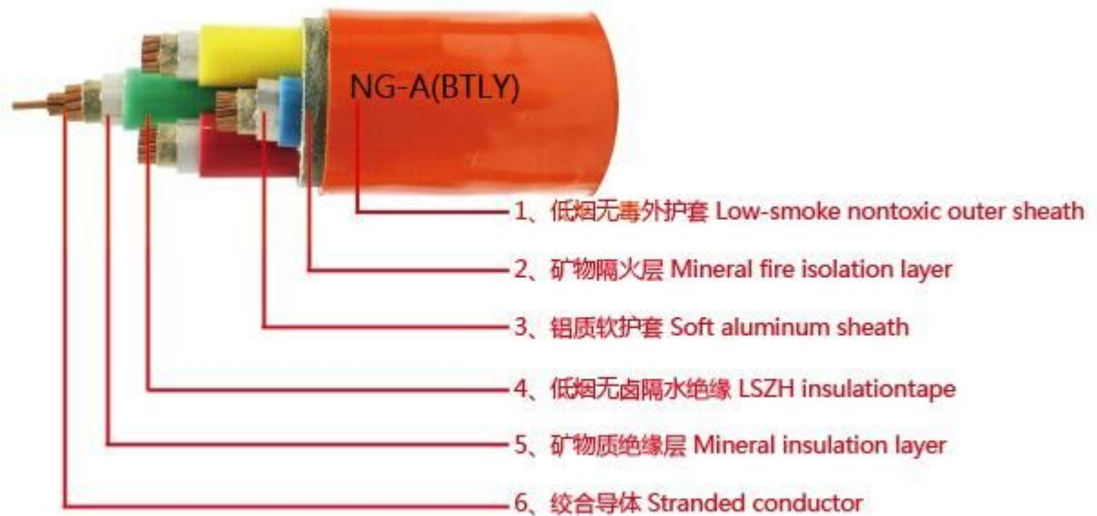
铝护套 ( 柔性 ) 隔离型防火电缆 Aluminum sheathed (flexible) fireproof cable of isolated type
