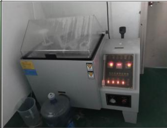
Salt spray test The machine test Android units metal not rusty.
