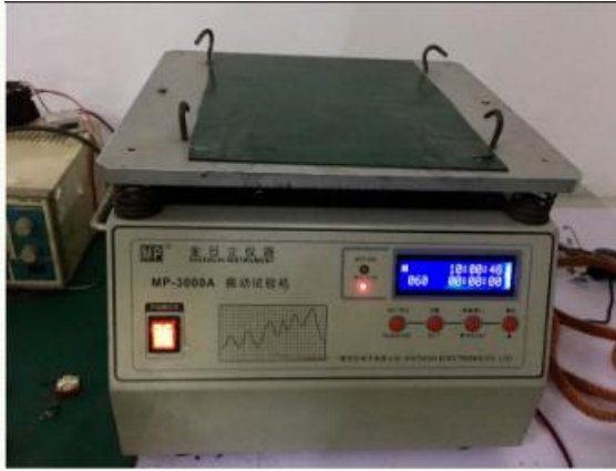
Micro vibration test Standard test: 60°, 65°, 70°, 75° The machine test Android unit spare parts if installed well.
