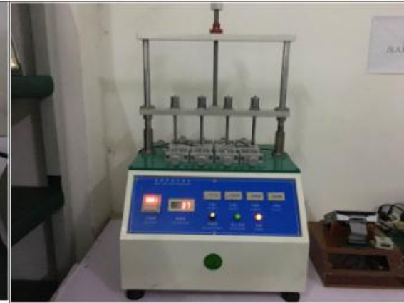
Buttons test The machine test Android units plastic buttons.
