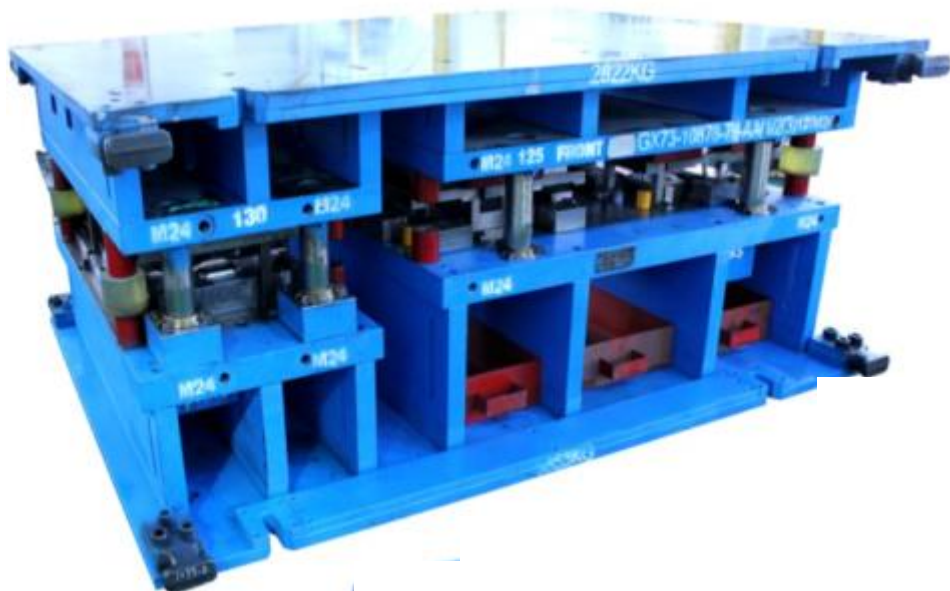
Jaguar project: transfer die Tool size: (2193+2112) \times 1462 \times 800
