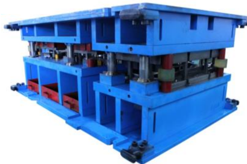
Jaguar project: transfer die Tool size: (2193+2112) \times 1462 \times 800
