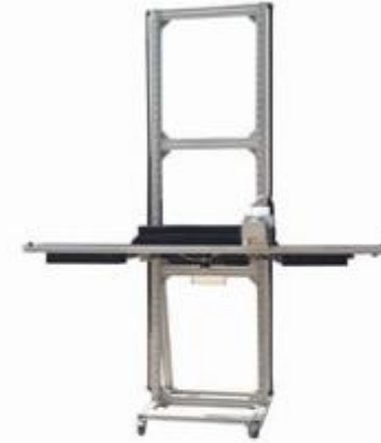
Year 2014, we developed lighter weight horizontal piezoelectric nozzle wall printer
