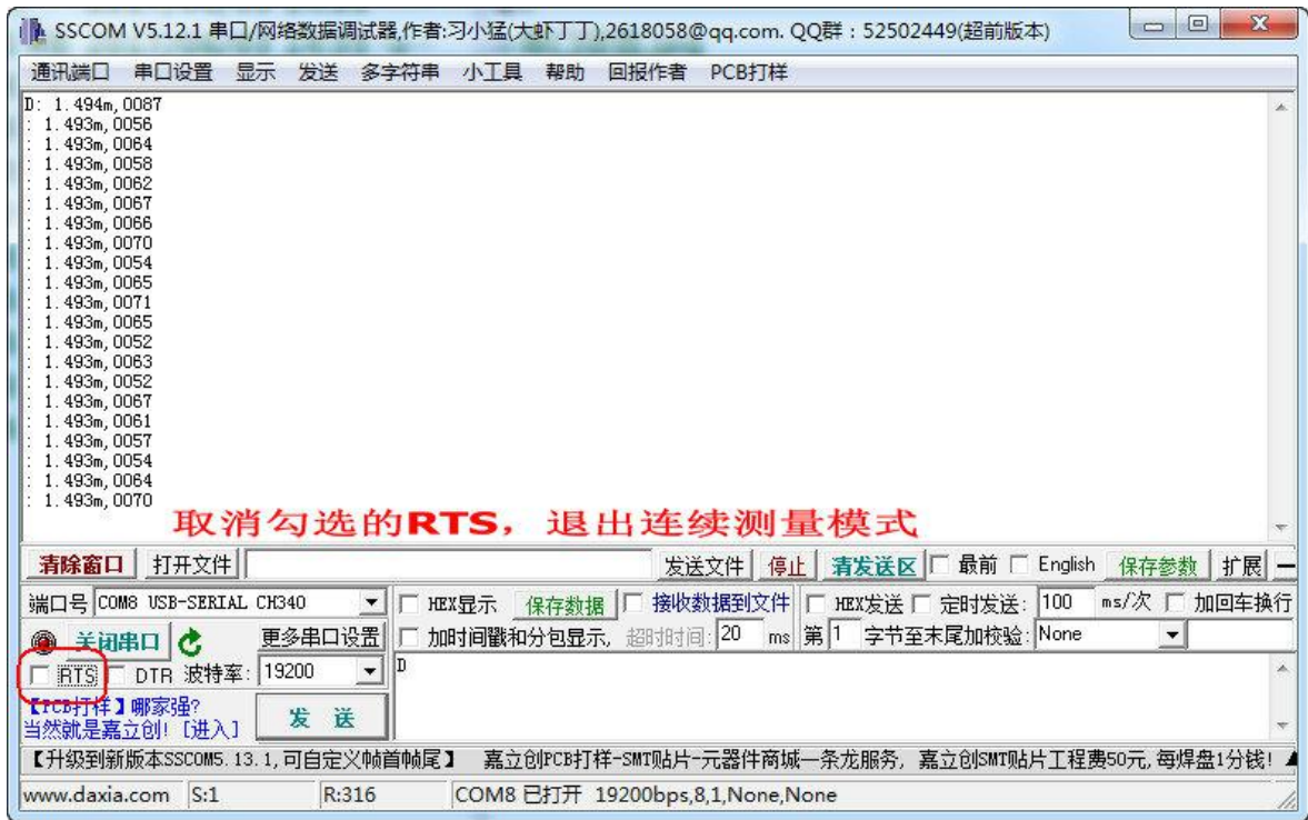
图 4-10 退出连续测量 Exit the Continuous Measurement Mode
