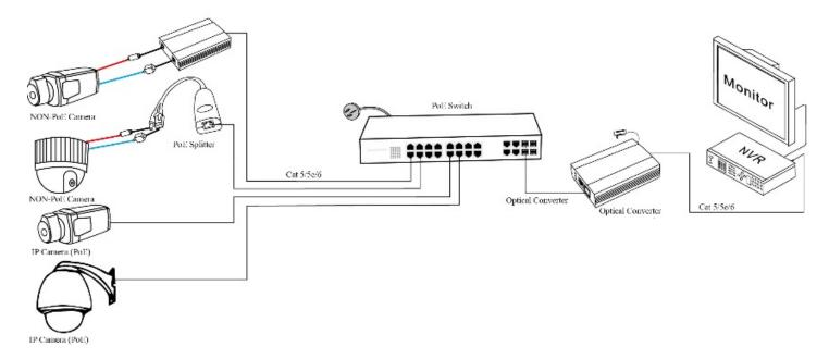
NT-29M16T4GC series is Management Ethernet switch with POE function, is dedicated to the application of video monitoring system and network engineering and design, to provide 16 Fast Ethernet ports and 4 COMBO ports (Gigabit UPLINK port: fiber and Ethernet port is optional).
