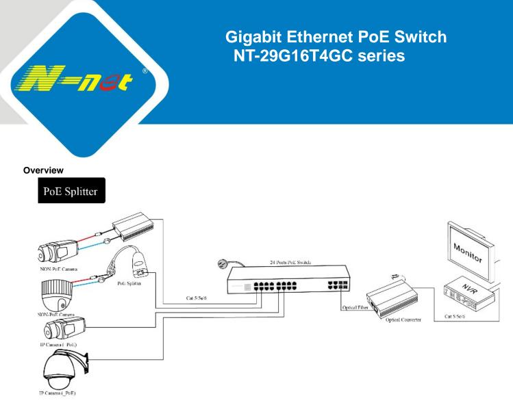
NT-29G16T4GC series is Gigabit Ethernet switch with POE function, is dedicated to the application of video monitoring system and network engineering and design, to provide 16 Gigabit Ethernet ports and 4 COMBO ports (Gigabit UPLINK port: fiber and Ethernet port is optional).
