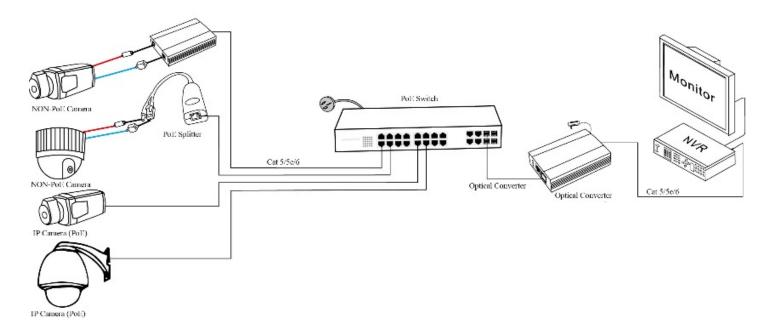
NT-2916T4GC series is Ethernet switch with POE function, is dedicated to the application of video monitoring system and network engineering and design, to provide 16 fast Ethernet ports and 4 COMBO ports (Gigabit UPLINK port: fiber and Ethernet port is optional).
