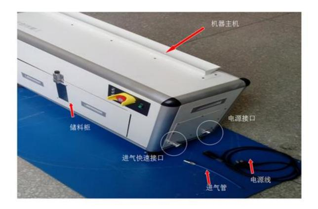
Site access power (AC210  $^{\sim}$  240V) and gas (0.4  $^{\sim}$  0.6MPa) can be used.
