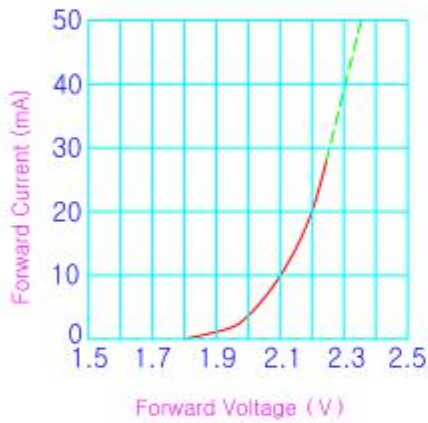
Forward Current Vs. Forward Voltage
