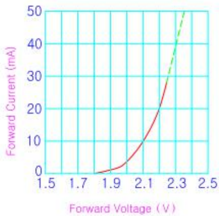
Forward Current Vs. Forward Voltage
