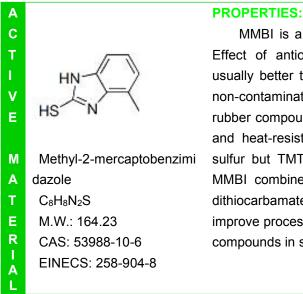
MMBI is a synergist for other antioxidants. Effect of antioxidants combined with MBI is usually better than that alone. It is a moderate non-contaminating antioxidant especially for rubber compounds contain ultra fast accelerator and heat-resistant rubber compounds with no sulfur but TMTD which is activated by MMBI. MMBI combined with CBS, MBT or thiurams, dithiocarbamate is an anti-scorcher and can improve processing safety and stability of rubber compounds in storage.
