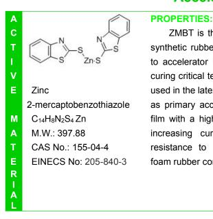
ZMBT is the accelerator for natural rubber, synthetic rubber and latex, performance similar to accelerator M, but weak effectiveness, high curing critical temperature(138°C). ZMBT mainly used in the latex, combined with ZDMC or ZDEC as primary accelerator. ZMBT vulcanized latex film with a high modulus. Meanwhile, no need increasing curing time also can get good resistance to compression set properties for foam rubber compound.
