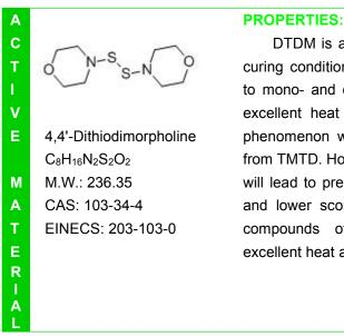
DTDM is a free sulfur donor under normal curing conditions. Compared to sulfur, it leads to mono- and di-sulfur cross-links and imparts excellent heat ageing properties. A blooming phenomenon will not occur, which is different from TMTD. However, acid ingredient in formula will lead to premature decomposition of DTDM and lower scorch safety. It applies to rubber compounds of low compression set and excellent heat aging properties.
