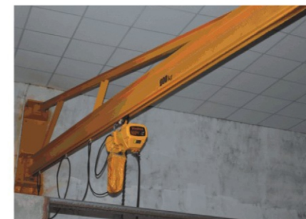
悬臂吊 Jib Crane
