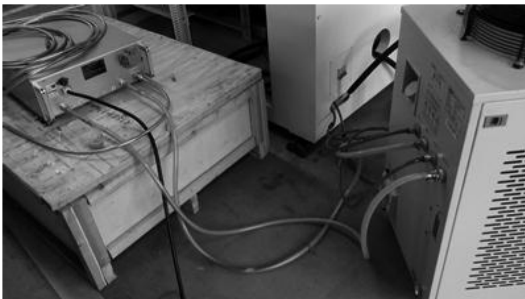
Figure 4-3 water cooler is connected with the optical fiber
