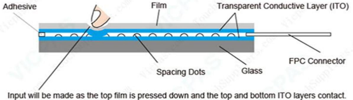
4wire and 5wire resistive touch screen is a two-layer structure, two materials (film or glass) with ITO are attached with a gap between them so that the ITO layers are facing each other. Touch input will be made as the top layer is pressed down and the two ITO layers contact. There are insulators called spacing dots between the top and bottom ITO layers. These spacing dots prevent unintended contacts (inputs) of the ITO layers when not pressed.
