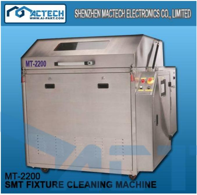
MT-2200 Fixture Cleaning Machine is use to clean grease, flux, dusts on the surface of all kinds of SMT fixtures, tray, reflow oven cooler and filter, wave-soldering oven claw, chains, and nets...etc.
