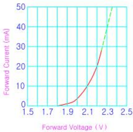
Forward Current Vs. Forward Voltage
