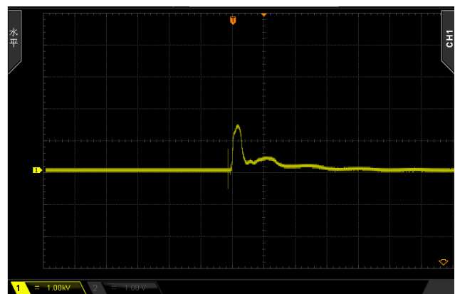
Output voltage waveform (differential mode 1.3KV)
