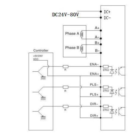
R=0 if VCC=5V R=1K(Power>0.125W) if VCC=12V; R=2K(Power>0.125W) if VCC=24V; R must be connected to control signal terminal.
