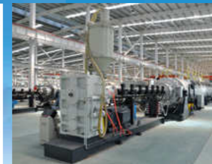
△ Introduced composite pipe production line with four layer 1000 mm steel wire mesh.
