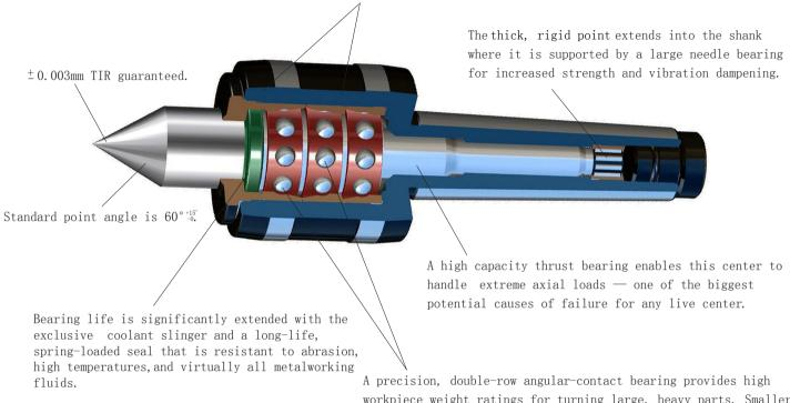
workpiece weight ratings for turning large, heavy parts. Smaller 2&3 MT models are not typically used to support very large workpieces so they are instead equipped with a single-row bearing that turns more freely and allows for higher speeds.
