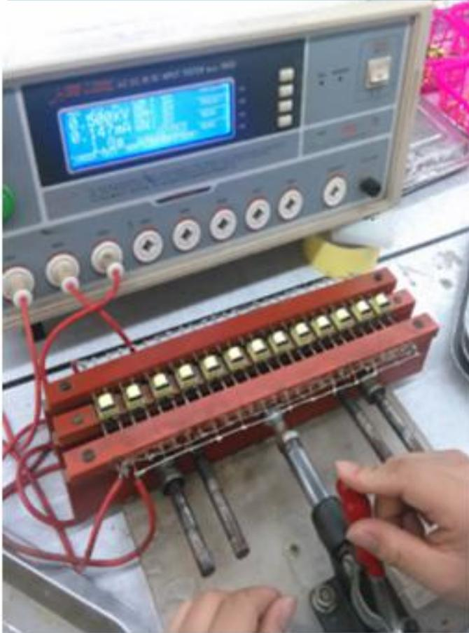
High voltage test: according to the new ICE76-3 standard to assess the insulation performance of the transformer, many design principles should be reconsidered, the processing plan should be changed accordingly, the experimental workload should be greatly increased.
