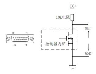
The controller provides 2-way digital output 1 9. The terminals are the MOS tube open-drain, the universal output amplitude is 24V 1A, and the maximum output is 40V 1A. In practical use, it is essential to connect a 10k pull-up resistor (as appropriate), as shown in the figure. For the digital output of every way, MOS
