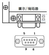
**Note**: when connecting motor and encoder, we need to notice that the A B phase signal of the encoder must match the connection of the controller to the motor. If the connection of the encoder is reversed, will cause the motor back and forth shaking uncontrollably, at this time, please exchange A, B encoder signal .
