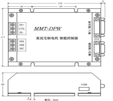
Note: The bottom of controller shell has  $4*\Phi5mm$  holes for installation and fixing, and installation can be conducted in the horizontal direction.
