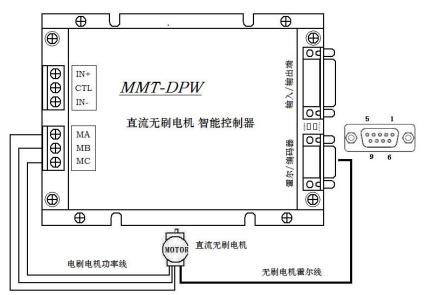
The controller output terminals A, B and C are used to connect the brushless motor
